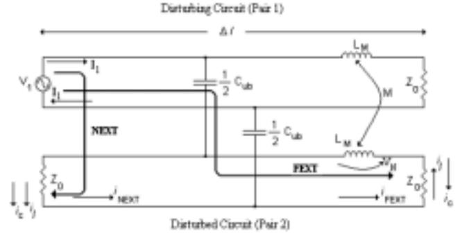
**Figure 5. Crosstalk coupling mechanisms (NEXT and FEXT)**
